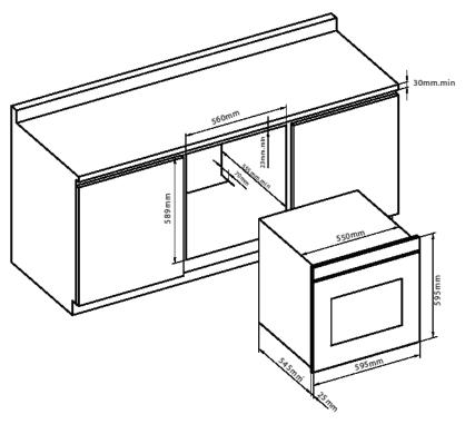
The figure opposite shows the ventilation and cut-out requirements for the installation of the appliance into a standard kitchen cabinet.
