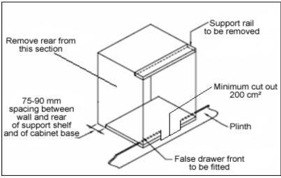
The figure opposite shows the ventilation and cut-out requirements for the installation of the appliance into a tall housing unit.
