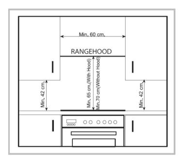
less than 70 cm. Refer to the range hood instructions for specific details before installation.
