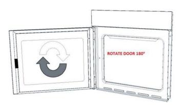
REFIT DOOR ON REQUIRED SIDE AND STAINLESS STEEL TRIM . SCREW OVEN INTO CABINET.
